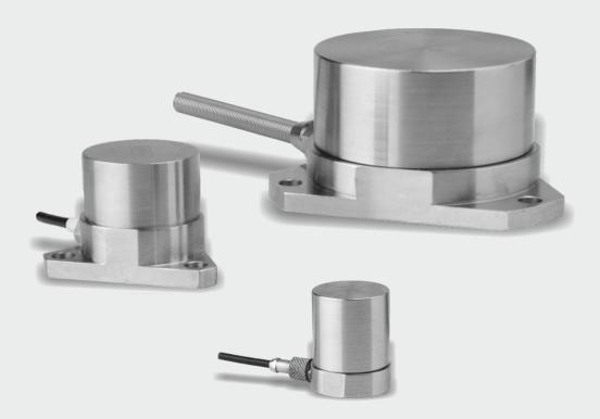
IPA Accelerometer utilizes the spring-mass system for generating a force proportional to the amplitude of the input acceleration to the base of the system. Force is applied to the piezoelectric (PE) element made of leadzirconate-titan ate (PZT) material that produces a charge output proportional to the force. The PE material is self-generating and does not require an external power source.
